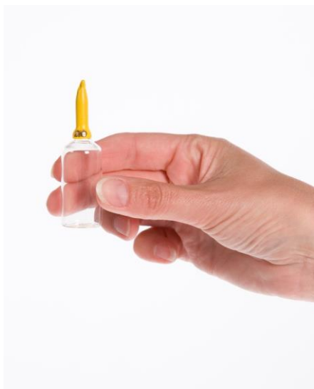
Figure 9: A NIST-traceable certified headspace standard manufactured by LIGHTHOUSE.
