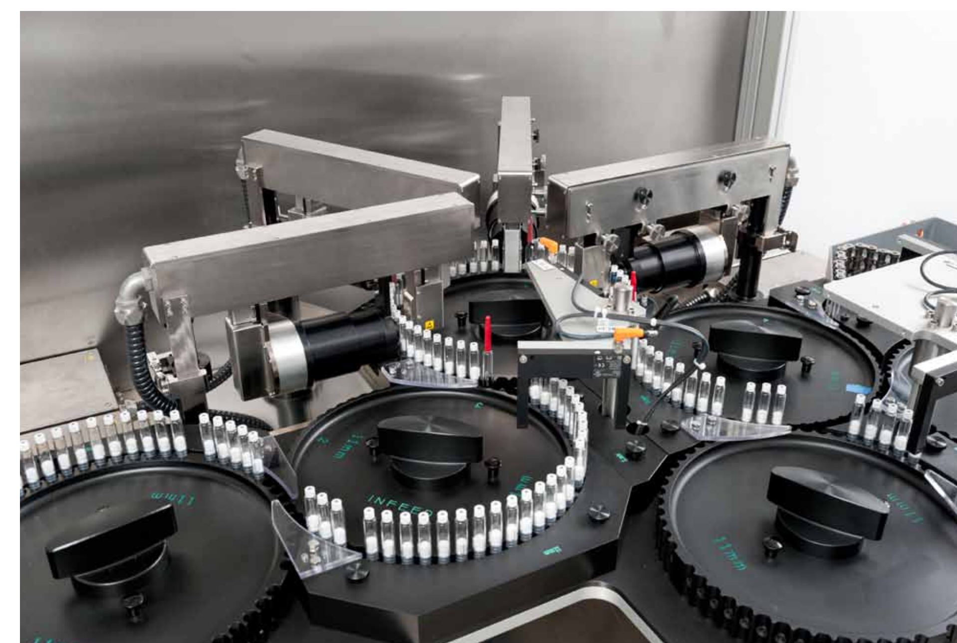
Photo 1 A close-up of the four oxygen sensor heads configured on a headspace inspection machine to inspect dual chamber freeze dried cartridges.
